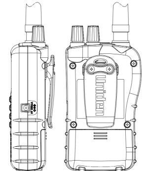
To make your scanner easier to carry when you are on the go, use the supplied belt clip. Use a Phillips screwdriver and the supplied screws to attach the clip to the scanner.
